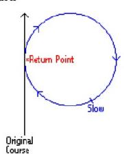
The Anderson Turn is a maneuver used to bring a ship or boat back to a point it previously passed through and is most appropriate when the point to be reached remains **clearly visible**.
