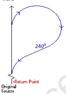
The Scharnow Turn is a maneuver used to bring a ship or boat back to a point it previously passed through and is most appropriate when the point to be reached is significantly further astern than the vessel's turning radius.
